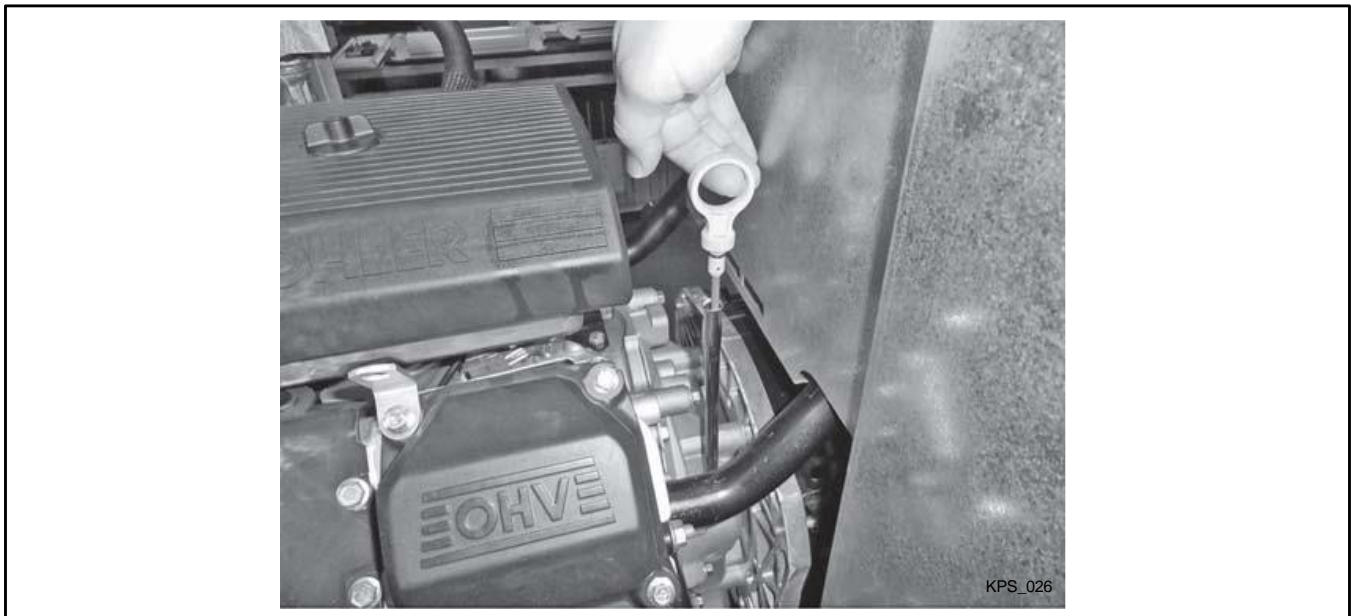
Figure 39 Oil Check (typical)
